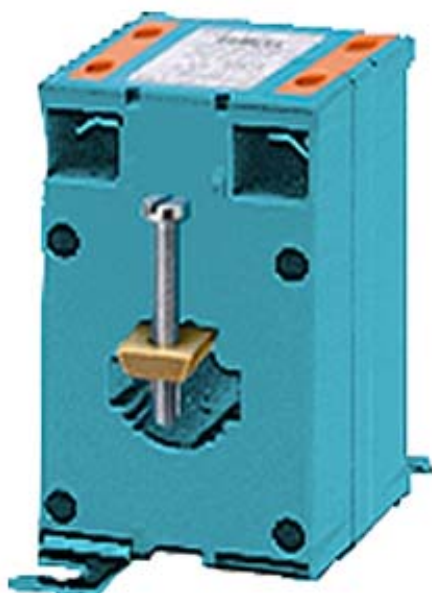
WINDOW-TYPE CURRENT TRANSFORMER, CLASS 3 50A/5A, 2,5VA PRIMARY CURRENT 50A, 2.5VA
