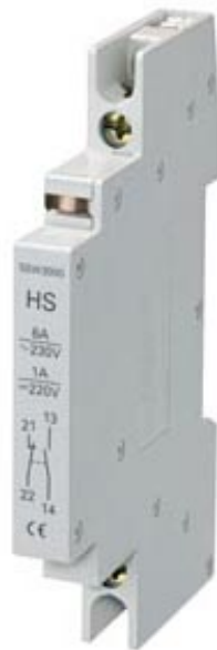
AUXILIARY SWITCH ATTACHABLE F. RES.CUR OP.CIRCUIT BR. 5SM1 T=55MM, 1NO+1NC
