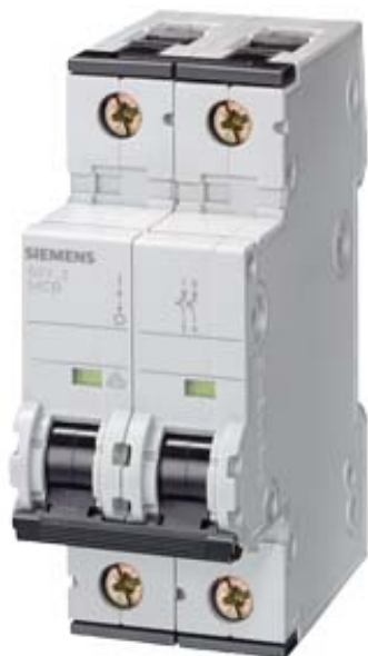
CIRCUIT BREAKER CURR. SENS DC 440V AC 400V 10KA, 2-POLE, B, 16A
