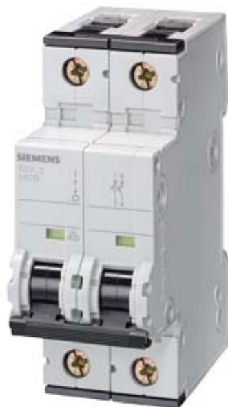
MINIATURE CIRCUIT-BREAKER UNIV. CUR. DC 440V AC /400V 10KA, 2-POLE, C, 63A FOR RAILWAY APPLICATIONS
