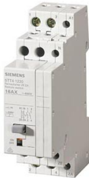
REMOTE SWITCH WITH 1NO WITH CENTRAL ON-OFF FUNCTION CONTACT FOR AC 230,400V 16A CONTROL AC 230V
