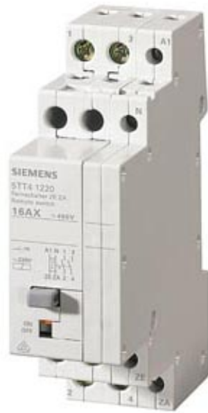
REMOTE SWITCH WITH 2NO WITH CENTRAL ON-OFF FUNCTION CONTACT FOR AC 230,400V 16A CONTROL AC 24V
