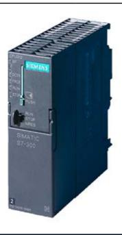
SIMATIC S7-300, CPU 312 CPU WITH MPI INTERFACE, INTEGRATED 24 V DC POWER SUPPLY 32 KBYTE WORKING MEMORY, MICRO MEMORY CARD NECESSARY
