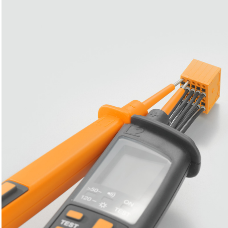
Maintenance through test tap
